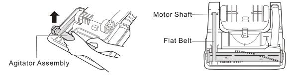
3 Place the flat belt onto the pulley of the new agitator assembly.
